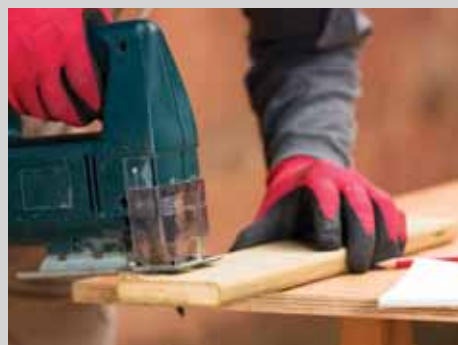
A jigsaw can be used to make curved cuts, straight cuts or fine detailed work in a range of materials
