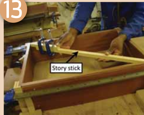
Fitting runners to cabinet side
