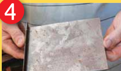
Make a 90° bend 20mm inwards on one of the 150mm sides
