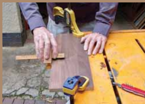
The one board must be 30mm longer, or wider than needed
