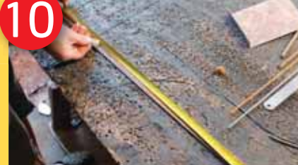
Determine the centre of the 1 250mm length of flat bar
