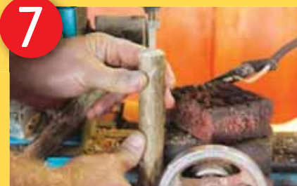
Drill an 8mm hole in an offcut piece of wood
