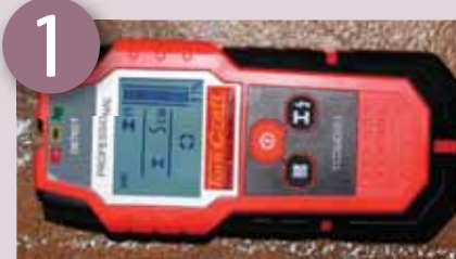
The metal detector indicated the depth of the water pipe at 5cm
