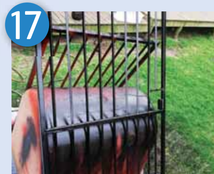
Paint with quick drying black paint
