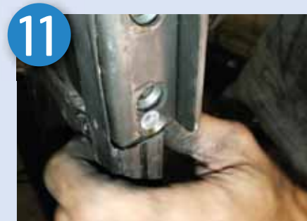
Fit slam lock mechanism
