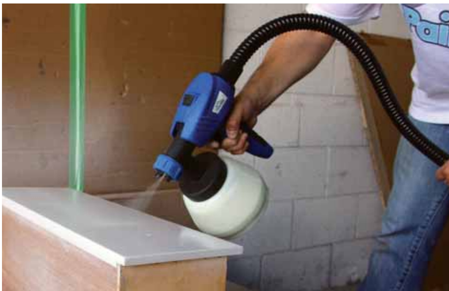
Hold the gun almost vertically downwards
