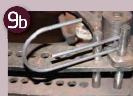
Bend 45° to prevent the toilet roll from slipping off
