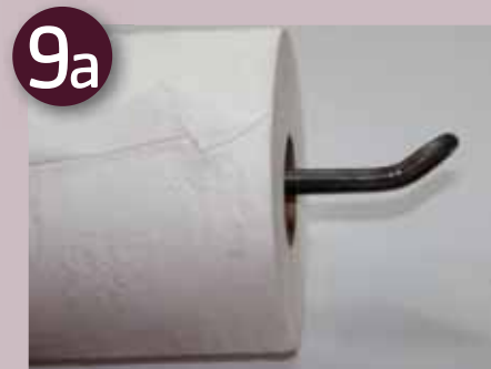
Bend 45° to prevent the toilet roll from slipping off
