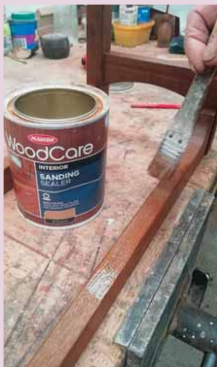
Seal the wood after it has been sanded and assembled in the frame
