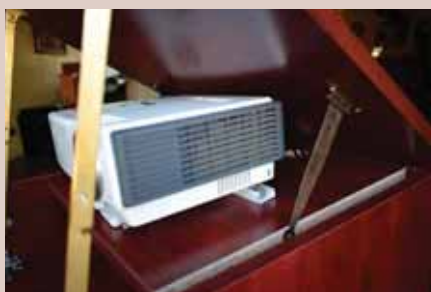
We used two tee hinges between the projector shelf and the cabinet lid
