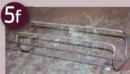
Cut the 6mm round bar and bend 90° on both sides
