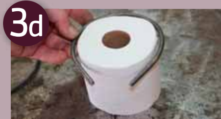
Cut two 350mm of 6mm round bar and bend a 135mm diameter circle
