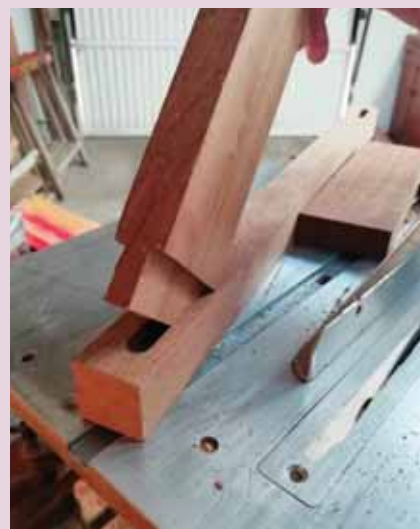
Cut the mortise using a plunge cutting router. The table saw can be used for cutting the tenon
