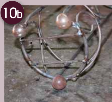
Weld the three cast iron balls on to form the feet
