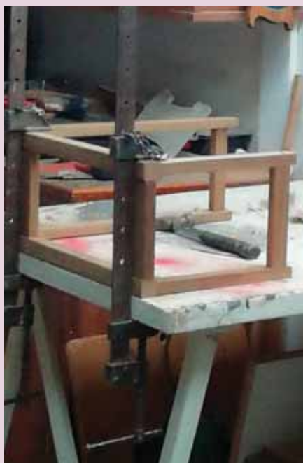
When you've assembled the construction and glued the joints in place, use a clamp to hold it all together while it dries
