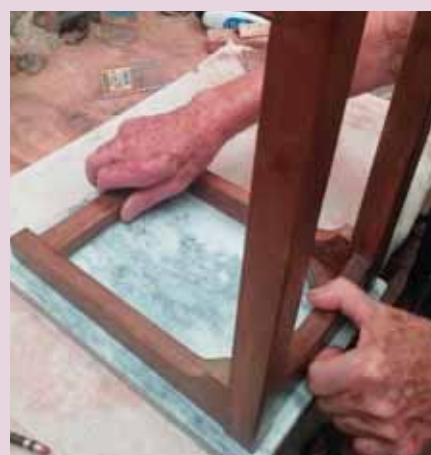
We used silicone to fix the marble to the wood frame
