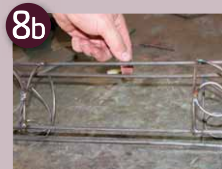
Weld the scrolls in place
