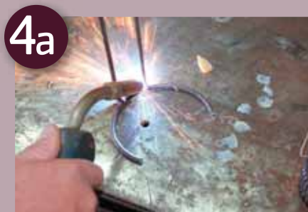
Cut two 350mm of 6mm round bar and bend a 135mm diameter circle
