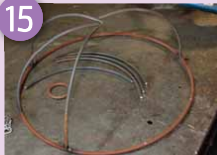
Weld up the curved sections
