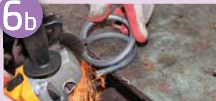
Cut the coil with a grinder (separate rings)
