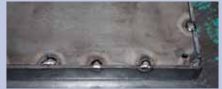
Spot welding is used when attaching sheet metal or angle iron or square tubing
