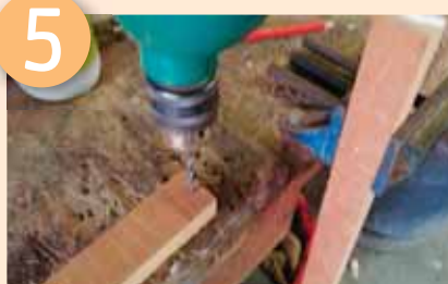
Drill pilot hole before joining with glue and screw
