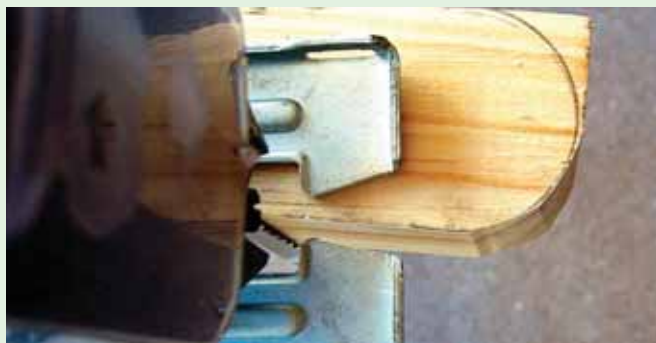
Fig. 6: Cutting the ends of the handle section
