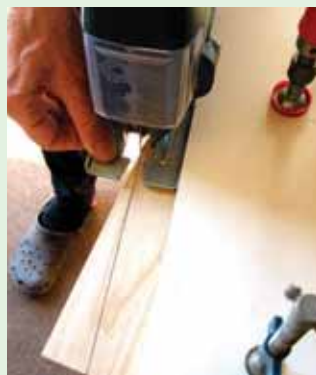
Fig. 8: Keep the jigsaw guide plate square to the guide piece
