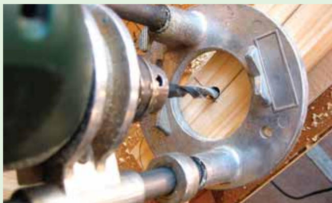
Fig. 4: Drilling the jigsaw pilot holes
