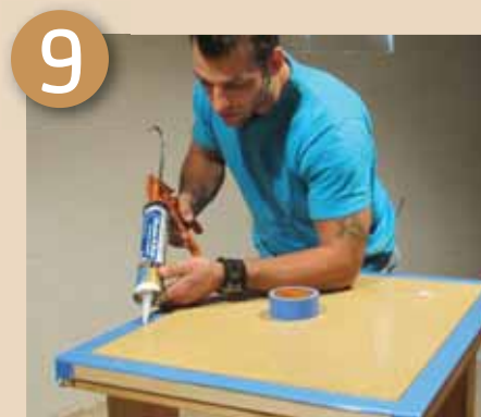
9 Run a silicone bead between the wood and cutting surface
