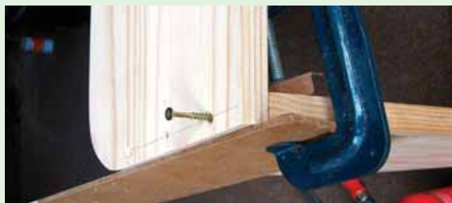
Fig. 12: Lining-up a side piece with an end piece
