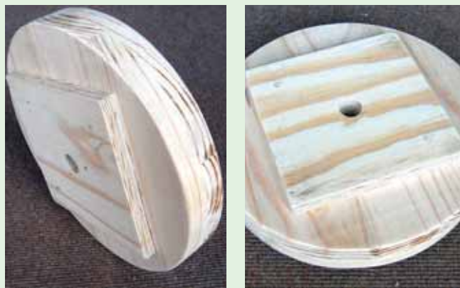
Fig. 11: The completed wheel assembly The 6 mm hole has been drilled out to 19 mm
