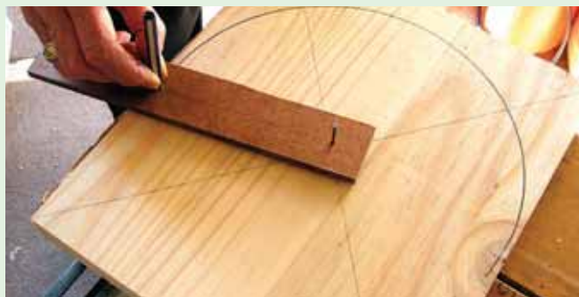
Fig. 3: Marking the wheel diameter
