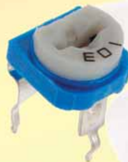
Variable resistor, called a potentiometer
