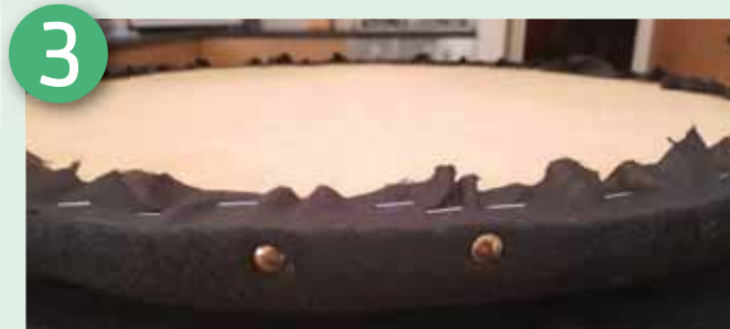
Drawing pins keep the foam in place
