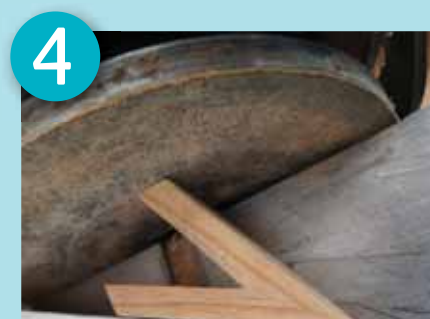
Use a second jig to grind the inside angles
