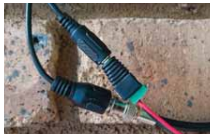
Analogue cameras are operated by a 12V power supply and co-axial communications cable
