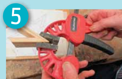
The rubberised clamp helps to fix the joins once glued
