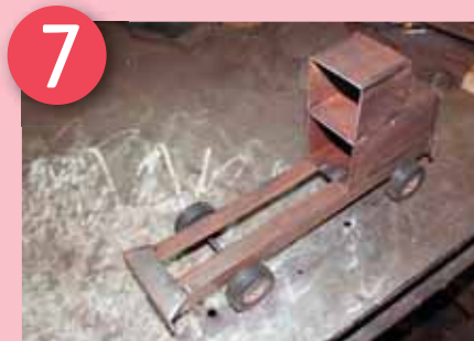
Two 130mm pieces of 6mm round bar are used for axles
