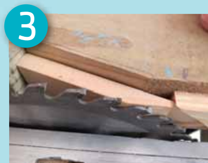
Use a jig to make consistent angles. Our machine required extra caution to operate safely
