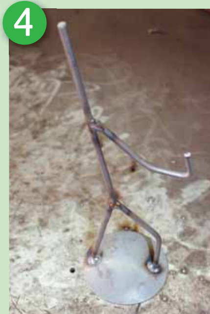
Weld the second arm in place
