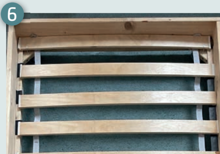
1. The dimensions of the bed we were gifted 2. Using a Kreg Jig, I drilled two pocket holes at each joint 3. I measured, marked and installed the slat support strips 4. Close up of the slat supports 5. To stabilise the frame further and create a base for the wheels 6. To keep the slats securely in place, I added L-shaped screws in all four corners 7. Two become one – how it looks with the bed slid under the main bed
