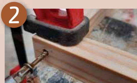
Clamp the loose components in place and fix the join with cold wood glue and the screw
