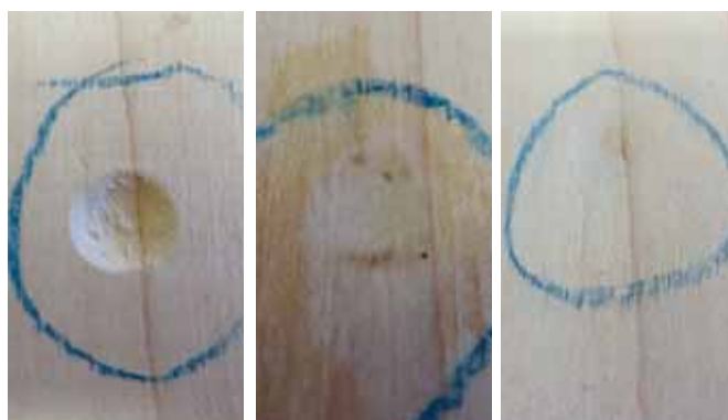
Dent in a piece of maple wood (peen hammered for illustration)
