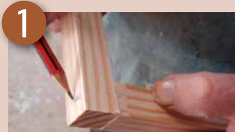
The horizontal must overlap the vertical. Mark the location of the drill-hole
