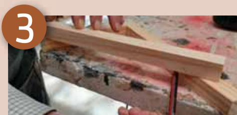
To determine angle to cut for the diagonal, place the timber across the horizontal and vertical portions and mark the underside, where it meets. That will be your cutting line
