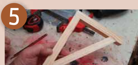
The first bracket will serve as a template for the remainder that you may need, based on the load bearing requirements
