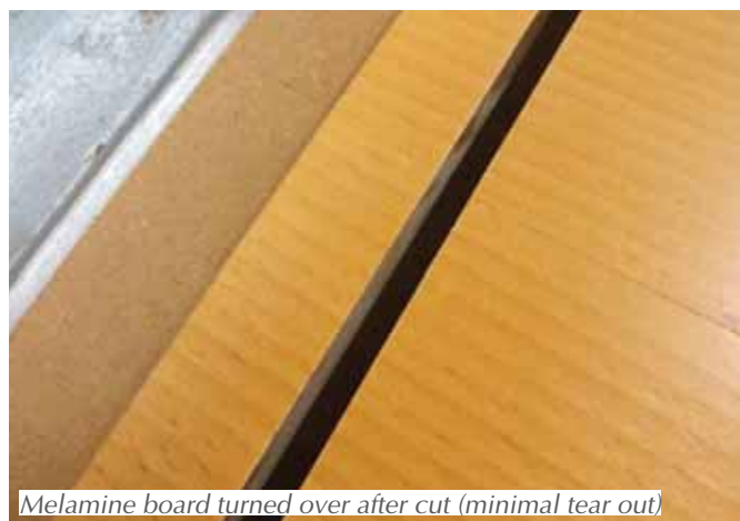
Board with 3mm MDF cutting melamine under the cut
